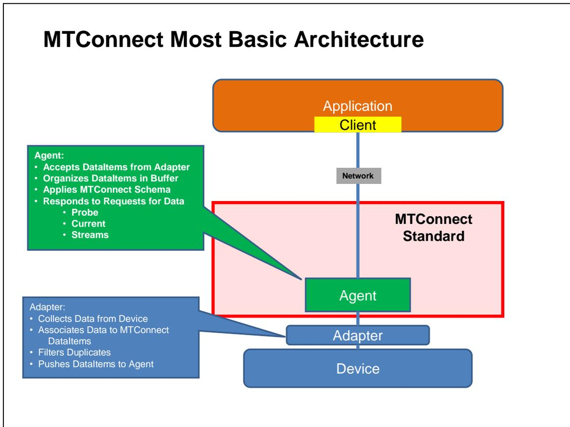
**Figure 1 – MTConnect Basic Architecture**
